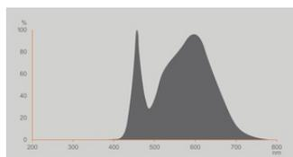
EPREL Data Spectral Diagram LEDr
